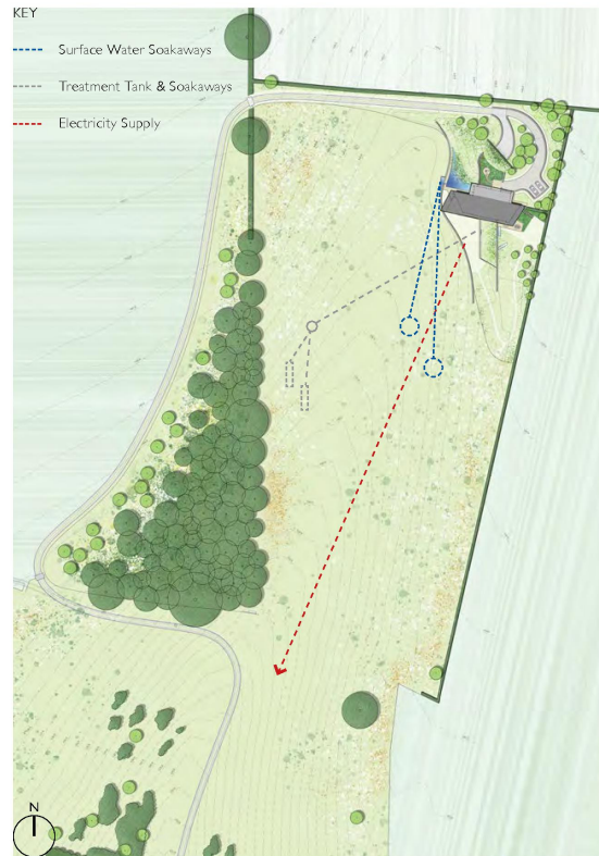
Foul Treatment Soakaway Field Drains
